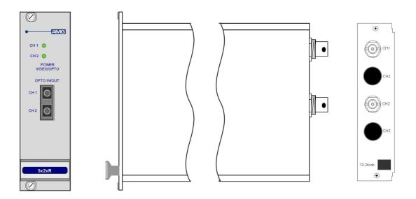
The **AMG5621R** is a DUAL rackmount system which provides two independent channels, each designed to transmit one video signal over one Multimode optical fibre. i.e. a total of two optical fibres.
